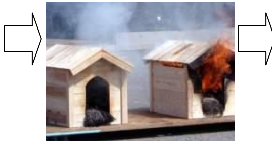
The house on the right has caught fire. The house on the left shows some carbonization, but the flames have not ignited.
