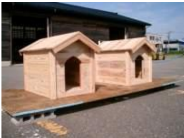
Right side: Regular lumber Left side : GP Fire Proof treated lumber
